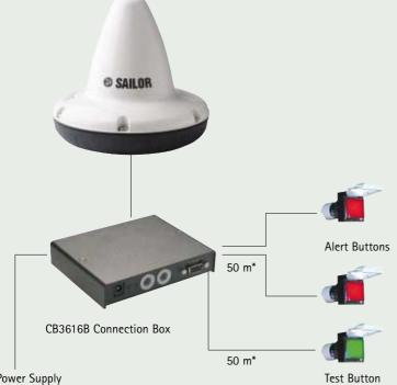
Power Supply Cable length up to 20 m: 10.5 – 32V DC Cable length up to 50 m: 16 – 32V DC \*Max 70 metres from Transceiver to Alert Buttons
